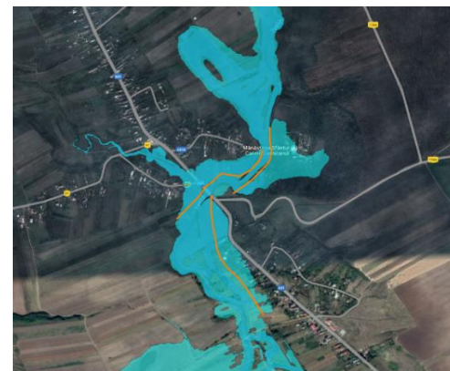
Dig nou, L = 1,8 km, h = 2m, Popanzalesti
